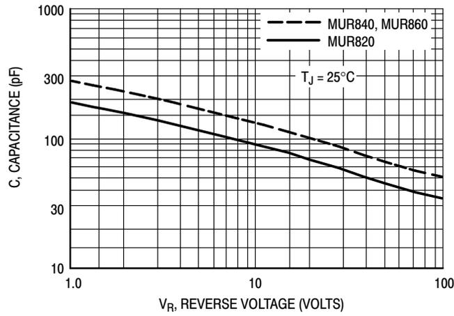
Figure 17. Typical Capacitance
