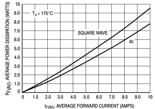
Figure 5. Power Dissipation
