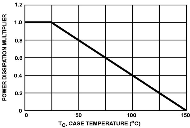
FIGURE 1. NORMALIZED POWER DISSIPATION vs CASE TEMPERATURE
