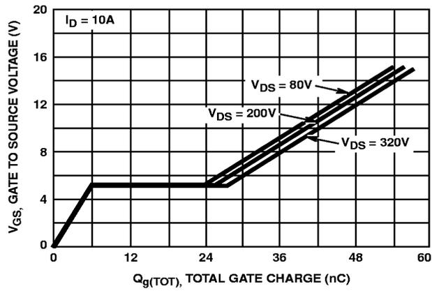
FIGURE 14. GATE TO SOURCE VOLTAGE vs GATE CHARGE
