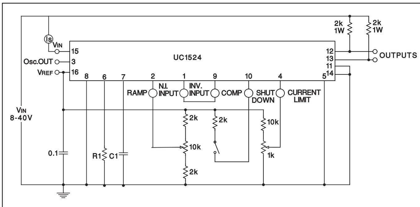
Figure 4. Open loop test circuit.
