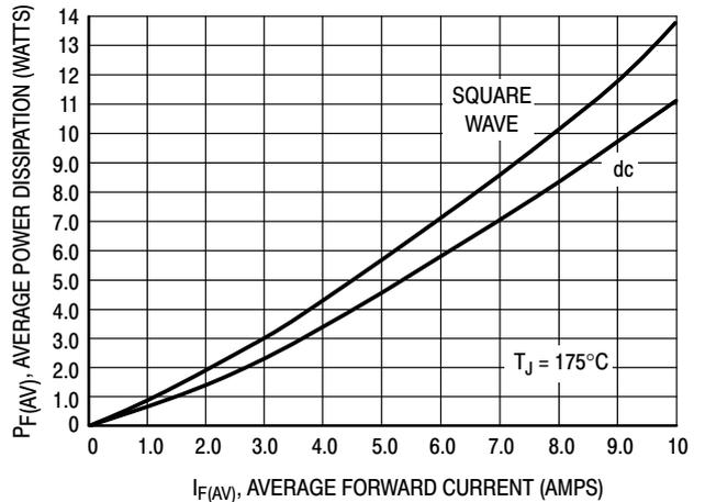
Figure 15. Power Dissipation
