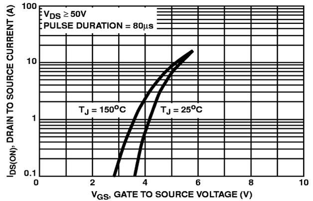
FIGURE 7. TRANSFER CHARACTERISTICS
