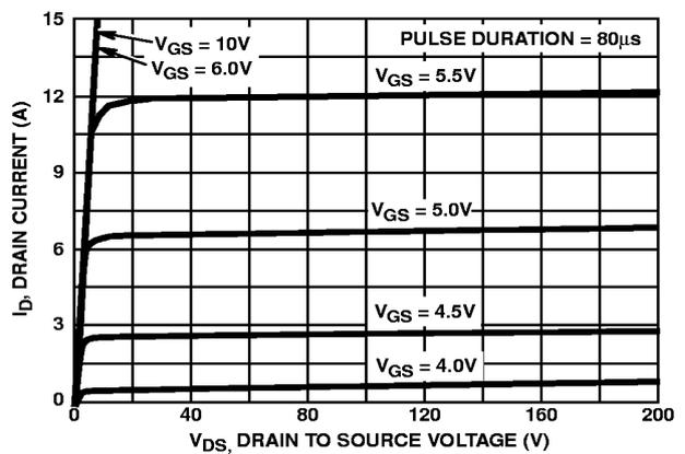
FIGURE 5. OUTPUT CHARACTERISTICS
