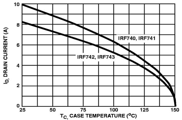
FIGURE 2. MAXIMUM CONTINUOUS DRAIN CURRENT vs CASE TEMPERATURE
