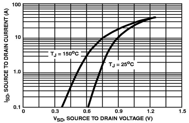
FIGURE 13. SOURCE TO DRAIN DIODE VOLTAGE
