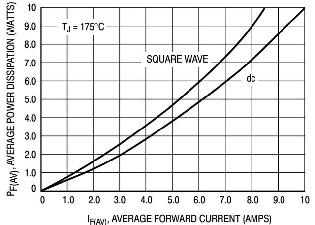
Figure 10. Power Dissipation
