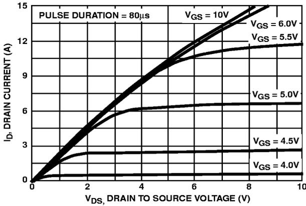
FIGURE 6. SATURATION CHARACTERISTICS
