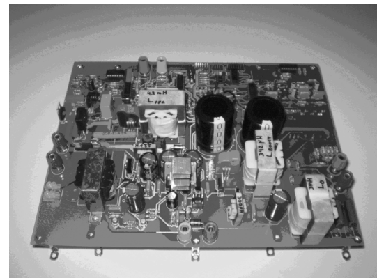
Fig. 12. PCB of the PFC converter and single-phase inverter.
