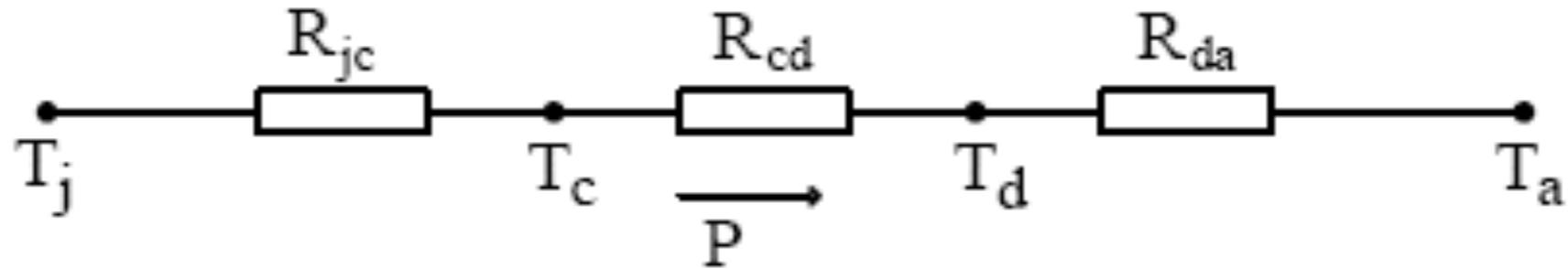
$$R_{ja} = R_{jc} + R_{cd} + R_{da}$$
